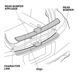
6. Insert the applicator into the soft sleeve. Starting from the middle and working outward, use the soft sleeve to smooth out the curved section of the rear bumper applique against the rear bumper. Move the soft sleeve in one direction only. Do not smooth the upper and lower sections at this time. If you see an air bubble, stop and gently peel up that section to work out the bubble. Work slowly and keep pressure against the rear bumper applique.
