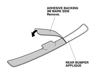
4. Spray the rear bumper applique with 3M protective tape application solution.
