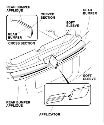
7. Using the soft sleeve, adhere the upper middle section and the upper side section of the rear bumper applique the same way.
