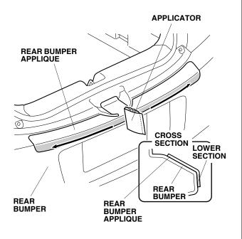
10. Using a shop towel, wipe the excess 3M protective tape application solution from the rear bumper applique. Allow the rear bumper applique to dry thoroughly.
